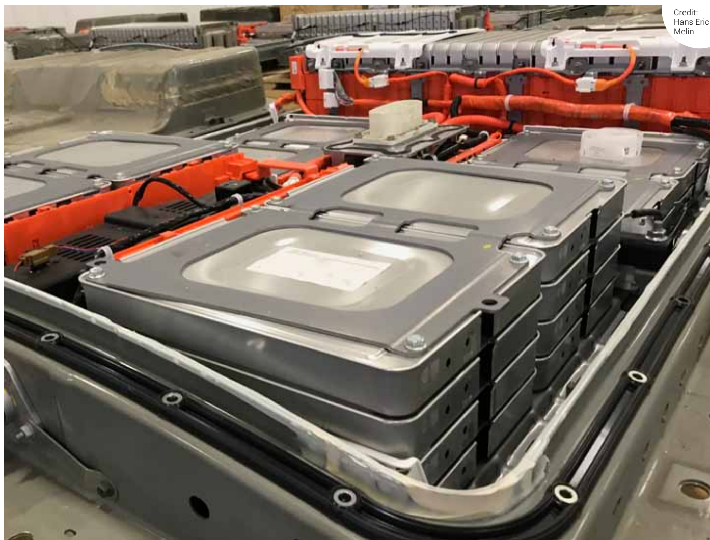
Nissan Leaf battery packs ready for disassembly. One of the most common battery types in second life applications
